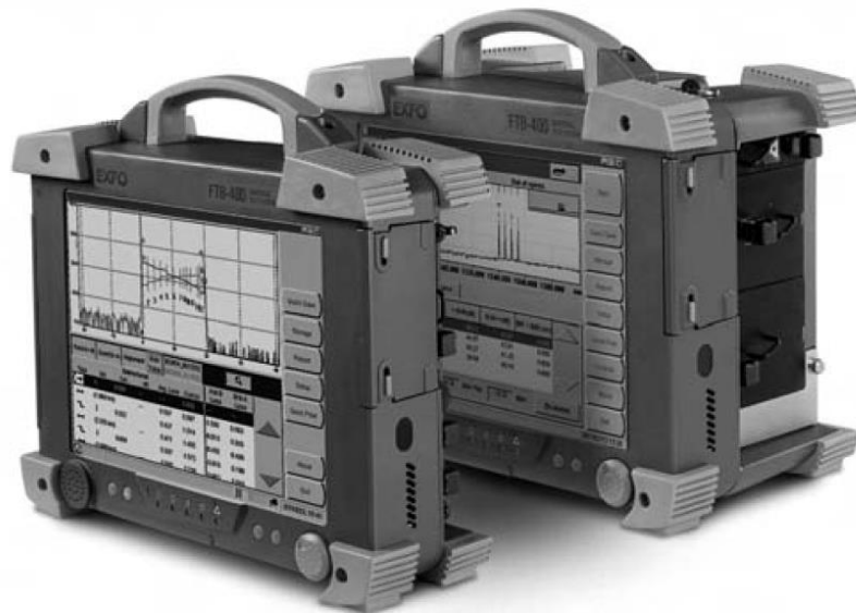
Figure 13.6. Portable OTDR for making measurements in the field. (Model FTB-400, photo provided courtesy of EXFO; www.exfo.com .)
