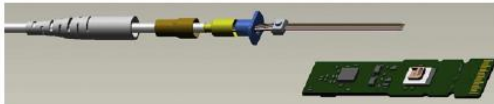
FIGURE 2.4 Basic building blocks of a pluggable transceiver [11].
