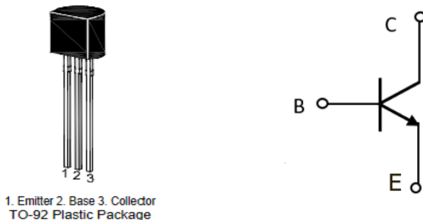
Fig. 1. 2N2222 BJT – pinout diagram
