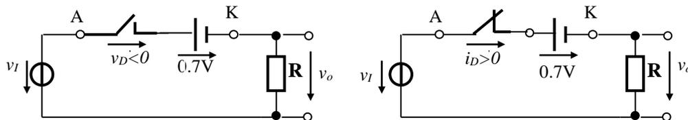
Fig. 5. Equivalent circuits for the DR two-port network in Fig. 4
