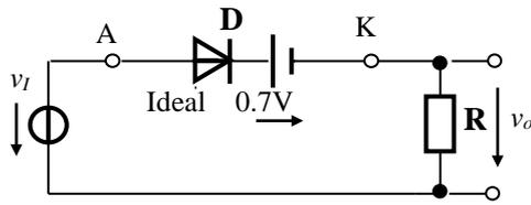
Fig. 4. DR two-port DR network, constant-voltage-drop model for the diode.
