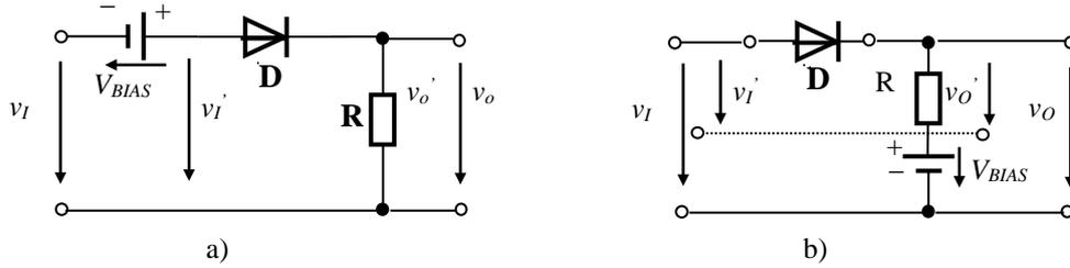
Fig.7 DR two-port network with a biasing voltage source:
