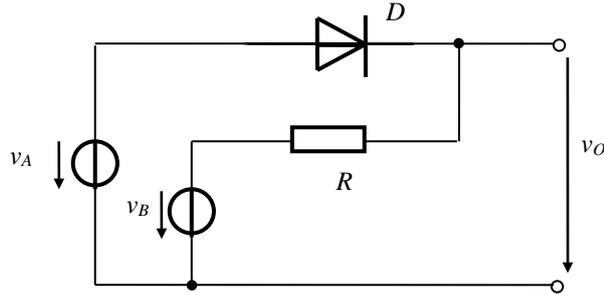
Fig. 9. Maximum three-port network.
