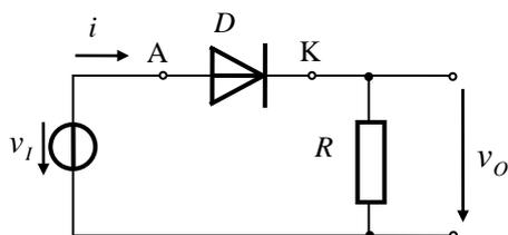
Fig. 1. Two-port DR network with output across R.
