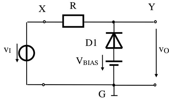
Fig. 12. Clamp two-port DR network with  $V_{Bias}$
