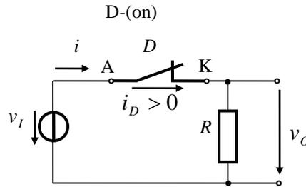
Fig. 2. b) Equivalent circuit for D-(on).
