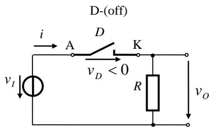
Fig. 2. a) Equivalent circuit for D-(off);
