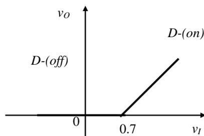
Fig. 6. VTC for the DR two-port network in Fig. 4.
