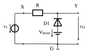
Fig. 12. Clamp two-port DR network with V<sub>Bias</sub>
