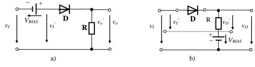
Fig.7 DR two-port network with a biasing voltage source: a) at the input port; b) common to the input and output port.
