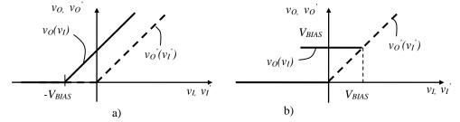
Fig. 8. VTC for two-port networks with a biasing voltage source: a) translation of the VTC along the  $v_I$  axis with  $V_{BIAS}$ ; b) translation of the VTC along the first bisector with  $V_{BIAS}$ .
