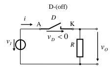
Fig. 2. a) Equivalent circuit for D-(*off*);
