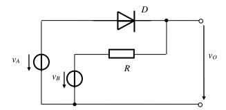
Fig. 9. Maximum three-port network.
