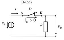
Fig. 2. b) Equivalent circuit for D-(*on*).
