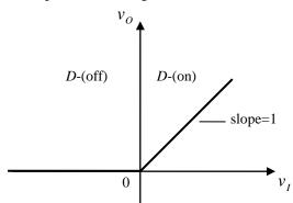
Fig. 3 VTC for the DR two-port network in Fig. 1.
