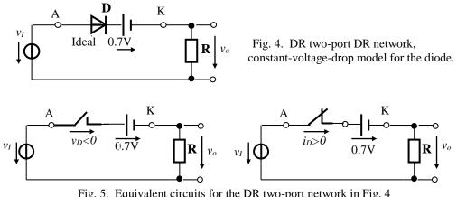
Fig. 5. Equivalent circuits for the DR two-port network in Fig. 4
